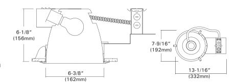
The 6" is designed for use in non-insulated existing ceiling or for existing insulated ceilings where insulation can be kept 3" away from all sides of the housing. It can be installed from below the ceiling.
